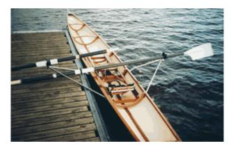
GIG2x EURO RACING Double Scull, Demo-boat, no use, length: 8,20 m, spread: 0,64 m, boat-weight: 43 kg only!, rowes weight: 55-90 kg,
