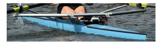
1x EURO RACING "ELITE" Midweight (new), 8,05 x 0,28 m, Carbon-Kevlar-Sandwich (Nomex), 03/2010, 65-80/85 Kg Rower Weight, ROWFIT WING RIGGER, ADIDAS Shoes, Size on demand.
