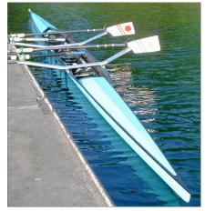
2x HUDSON RACING DOUBLE "ELITE", Lightweight, former spare Boat from Worlds, 45-64 Kg Crew Weight, 9,40 x 0,29 m, Carbon-Prepreg-Sandwich, ROWFIT WING RIGGERS, ADIDAS Shoes, Size on demand, Color: white,
